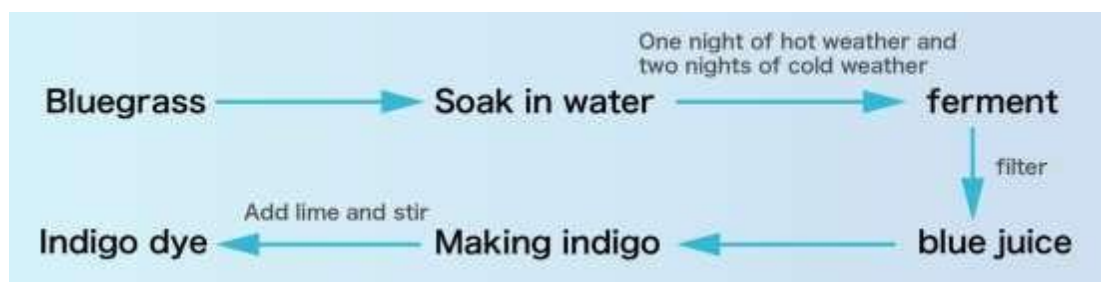
Figure 2 : The Process of Making Indigo (Source: Produced by Author)
