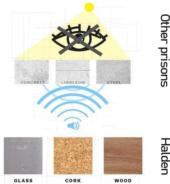
Figure 7: Materials that absorb noise and allow natural light
