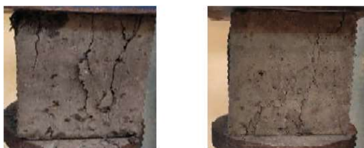
Fig. 3 Failure Pattern of Cube specimens
