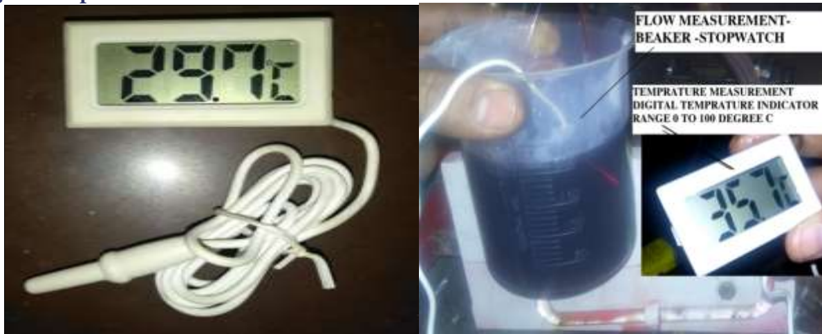
Fig. no. 7. Temperature Sensor with Mass flow and temperature measurement set up
