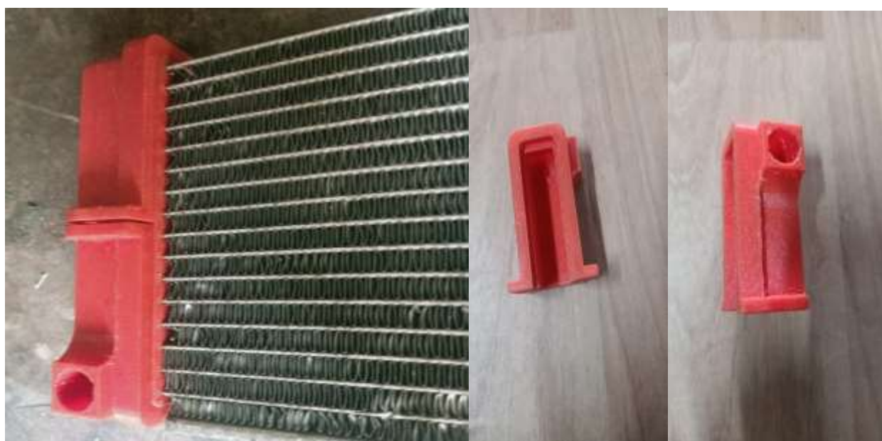
Fig.no.5 (a) flat plate heat exchanger (b) 3D printed micro-channel fin holder
