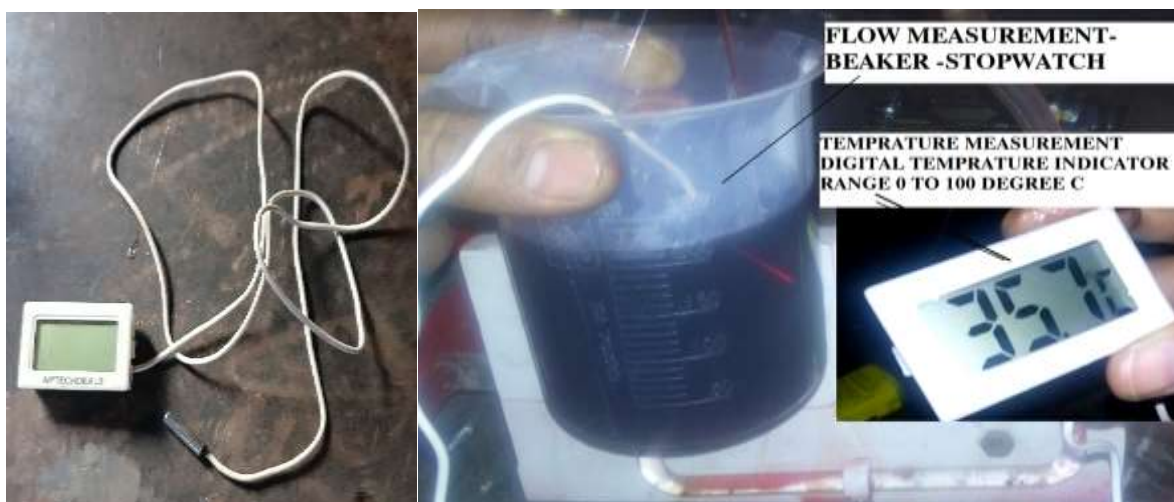
Fig.no. 9. Temperature Sensor with flow measurement
