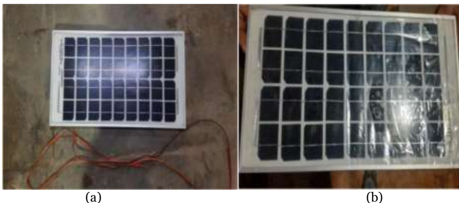
Figure 3: Gallium arsenide solar cell (a) Prior to encasing (b) Following encasement.
