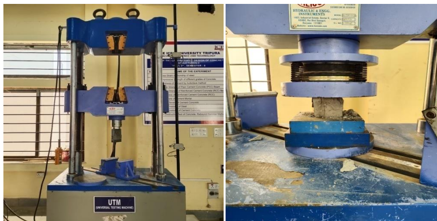
Fig 4.2: Testing of Compressive strength of the light weight AC cubes
