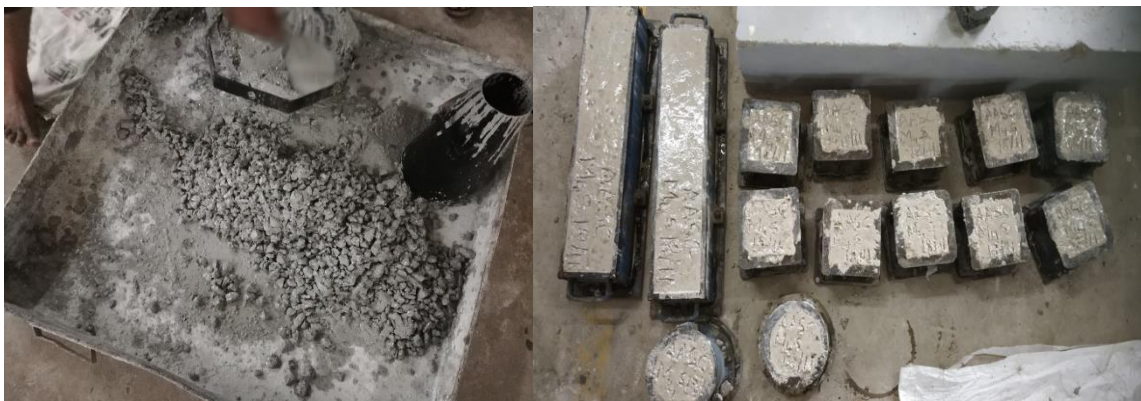
Figure 3 Mixing & Casting of Specimen
