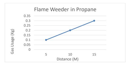
An analysis was conducted to assess the efficiency of propane gas usage in flame weeding applications. Gas usage, measured in kilograms, was analyzed in correlation to the corresponding distance covered, measured in meters. The results of the analysis showed: 0.1 kg of propane gas was used to cover 5 meters, 0.2 kg was used to cover 10 meters, and 0.3 kg was used to cover 15 meters.
