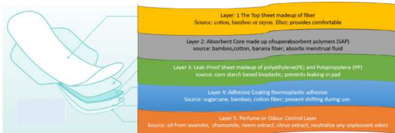
Fig 2: Construction of Eco-Friendly layer design for Biodegradable Menstrual Hygiene Products in sanitary pads
