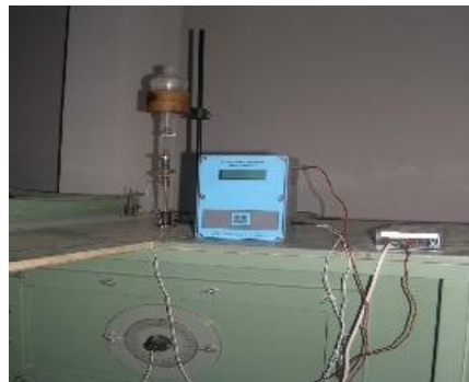
Fig 6. Complete Hot wire Smoke Visualization Set-up
