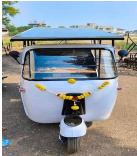
Fig 9. Prototype of Solar Powered Plug-EV
