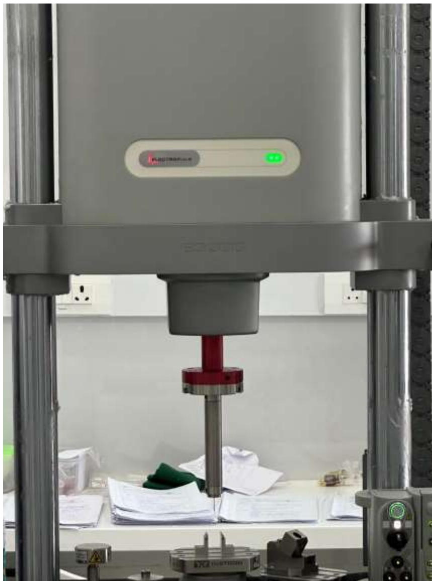
Fig 4. Flexural strength using Universal Testing Machine
