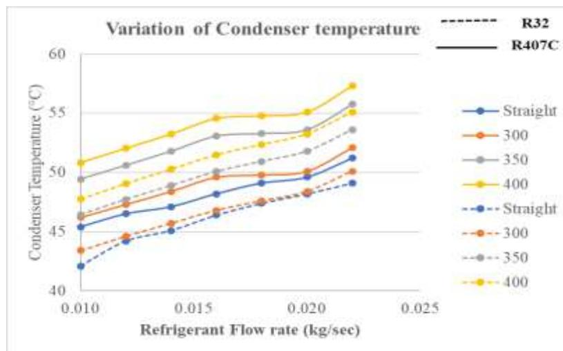
**Figure 3: Variation of Condenser Temperature**
