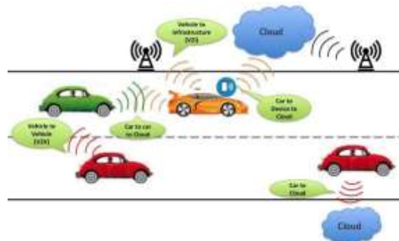
Fig :2: Types of vehicle-to-everything communication supporting connected vehicles
