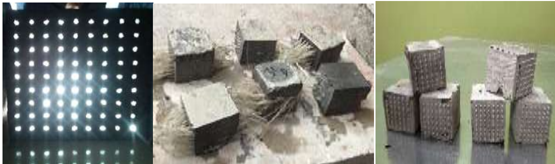
Fig.3. Process of production of Optical fibre base transparent concrete (Adopted from Salih, 2014)
