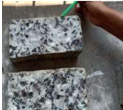
Figure 1. Visible evidence of chlorine diffusion
