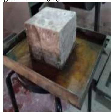
Figure 3. Water Absorption of cubes by capillary action
