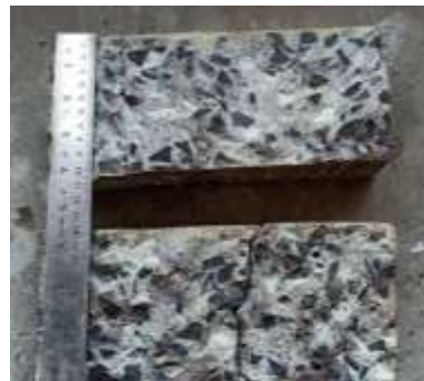
Figure 2. Measurement of Penetration depth of chlorine in concrete
