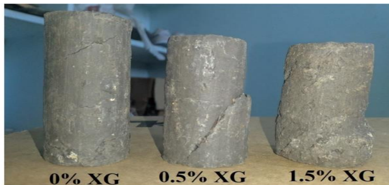
Figure 4.7: Failure Patterns of Xanthan Gum treated clayey soils.
