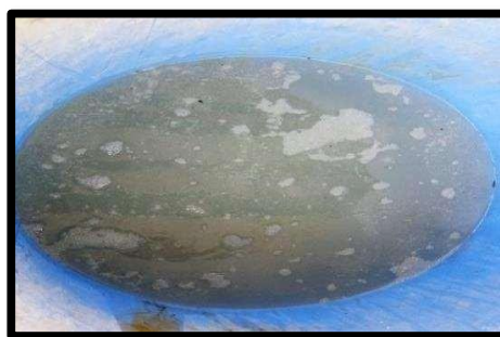
Figure 2.3.5 Concrete cube immersed in 5% in H 2 SO 4
