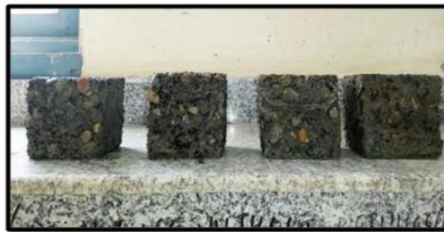
Figure 3.7 Showing spalling in cubes after sulphuric acid attack
